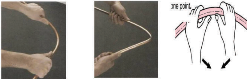
Manual bending of pipe
