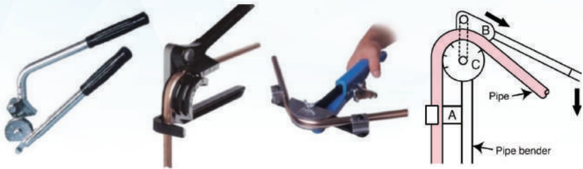
Bending by pipe bender
