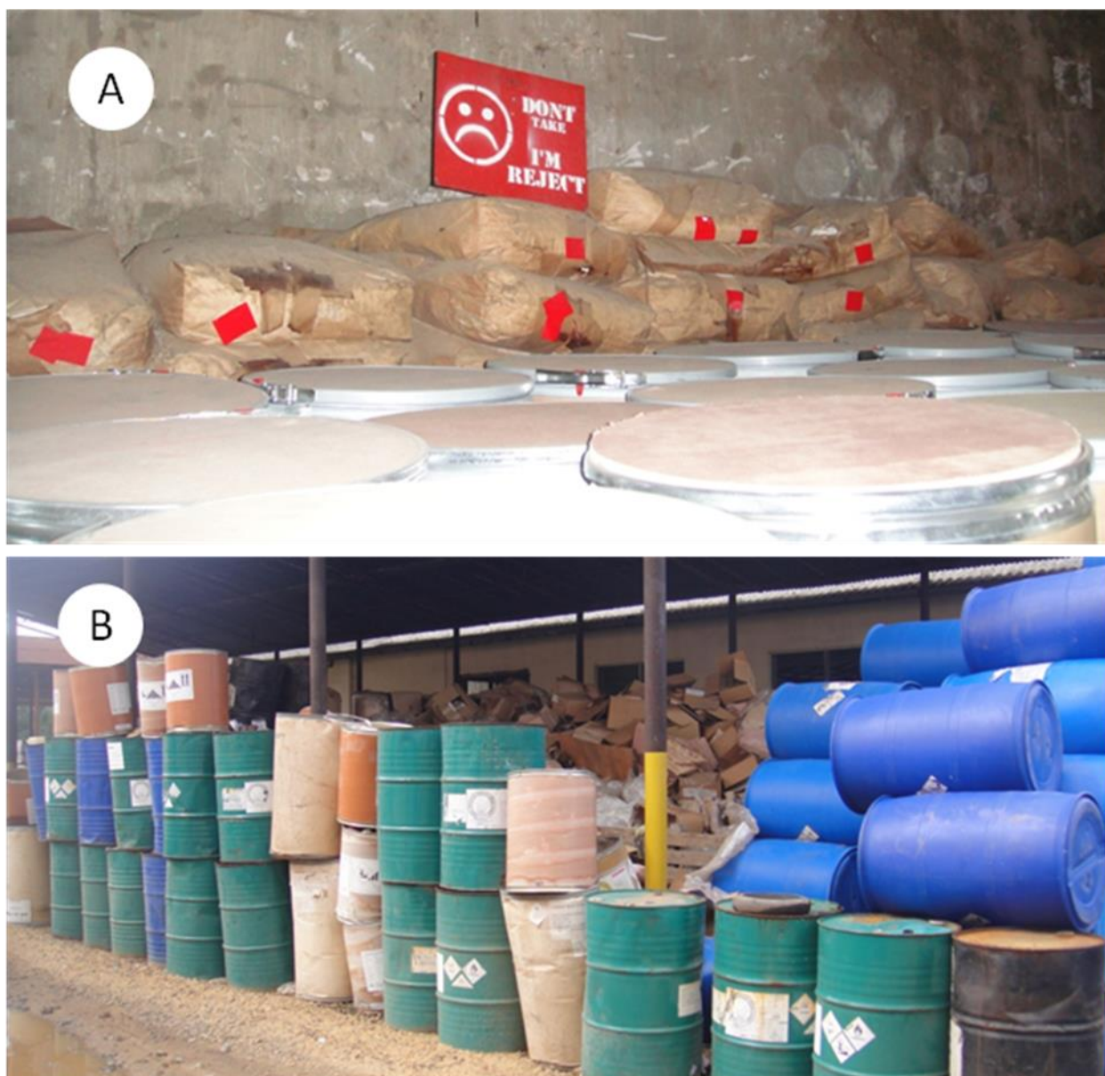
Figure 10: The nature of non-POPs pesticides waste for disposal: (A) A stock of obsolete pesticide formulations; (B) A stock of pesticide contaminated waste including bulk containers. Location: Ceylon Petroleum Corporation (Agrochemical Function), Kollonnawa, Date inspected: 17.02.2012 (Photos by J.A. Sumith).
